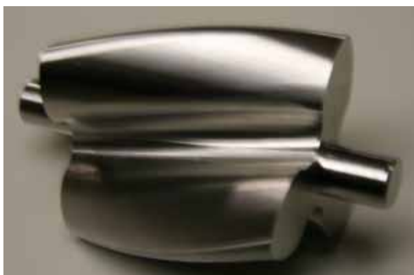
Three teeth rotors - 5-Axis Simultaneous machining
